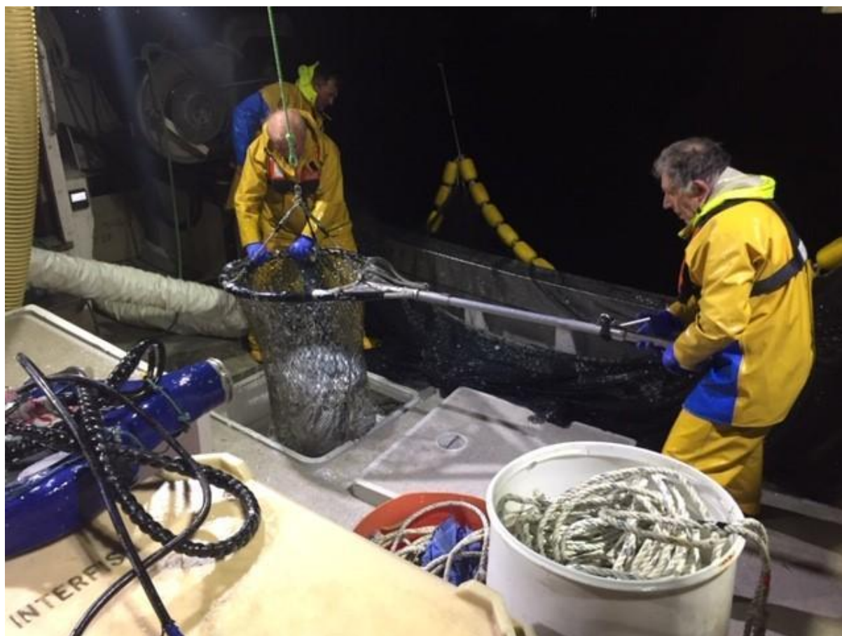
Figure 7. the alternative system to pumping the catch is brailling the catch aboard the vessel. This may be used at the end of the catch process to clean the small reminder of fish in the net. Source: CU UK.
