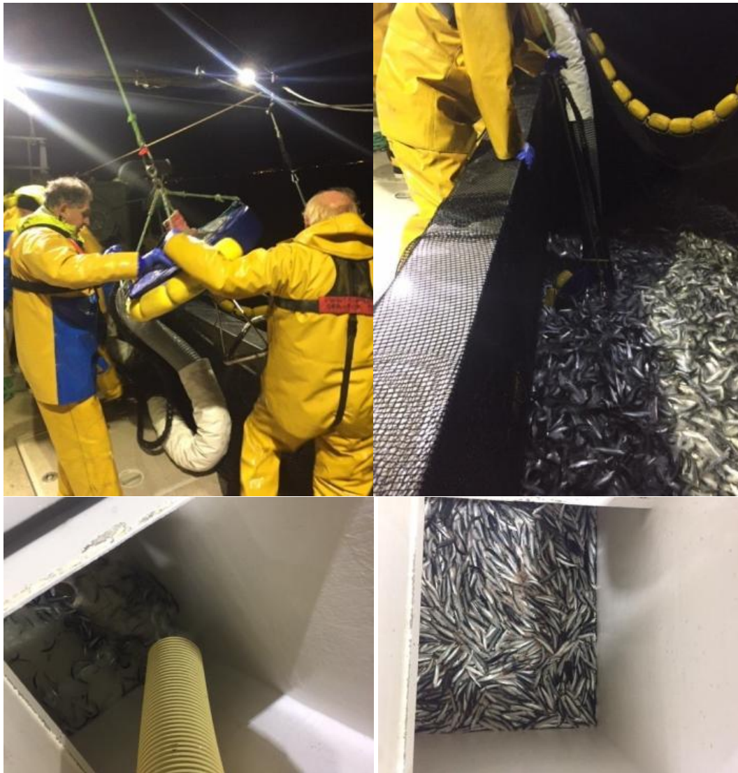
Figure 6. Pumping the catch aboard a CSMA vessel into the vessel integrated holds. Source: CU UK.
